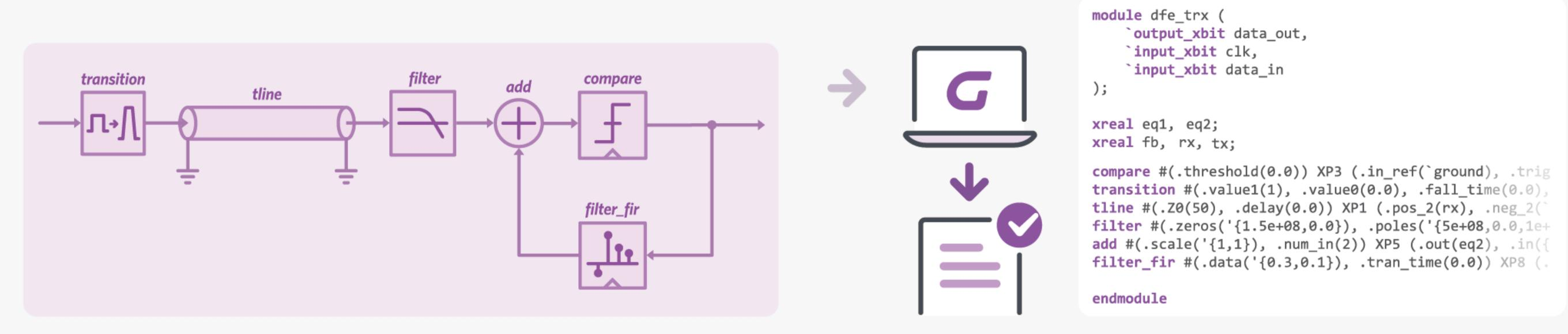
Draw model schematics with XMODEL primitive symbols
